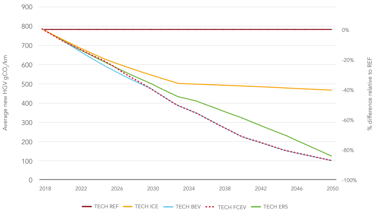
Figure 10. Impact of the ZEV scenarios on EU CO 2 emissions from the average new HGV in each scenario.
