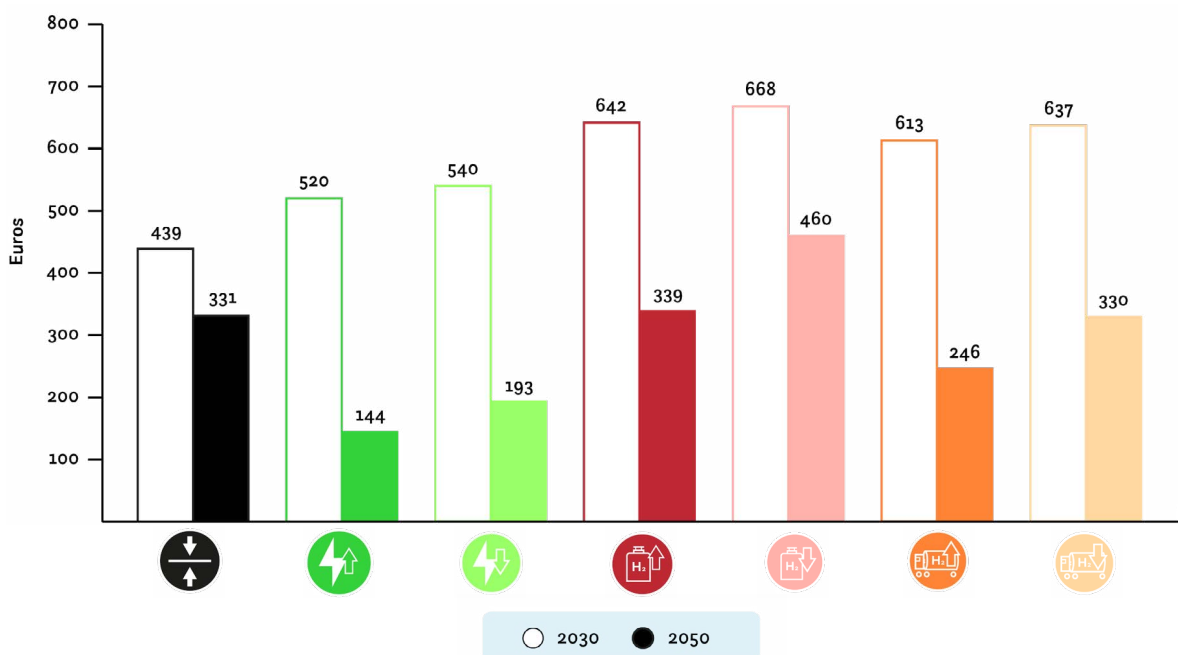
Figure 7: Average annual heating bills (in €) per household in Europe in six decarbonisation scenarios compared to the baseline
