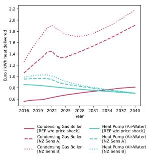
Figure 3-9: Running total cost of ownership developments for selected technologies and scenarios, EU average, 2016-2040, in €/kWh of heat delivered.
