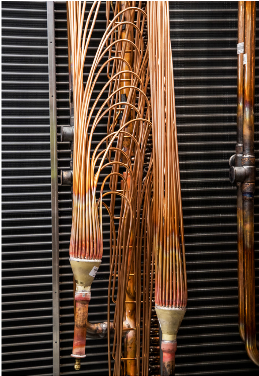
Villapaiera (Italy). Detail of the copper pipes in a heat pump produced by the Clivet company in Villapaiera in the province of Belluno.
