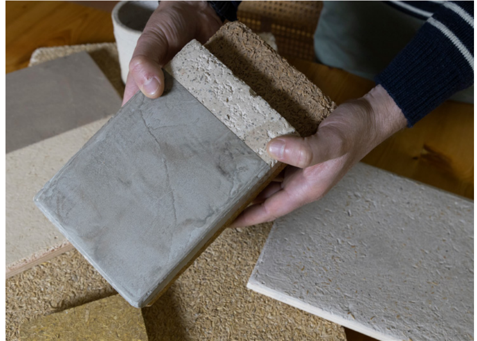
Andorno Micca (Italy). Insulation material for homes made from rice by-products by the Rice House company.
